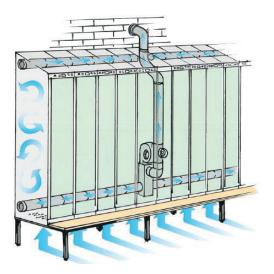
Type C, Blika mechanical drying ventilation. Re-circulation
